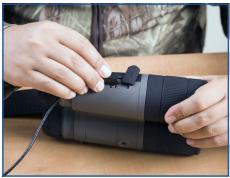
Insert the microUSB plug in to the microUSB media port.
