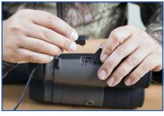
Depending on the device you have, you would either lift the rubber media port to expose the media slots. Or unscrew the media port cap if using with the ATN OTS-X HD.
